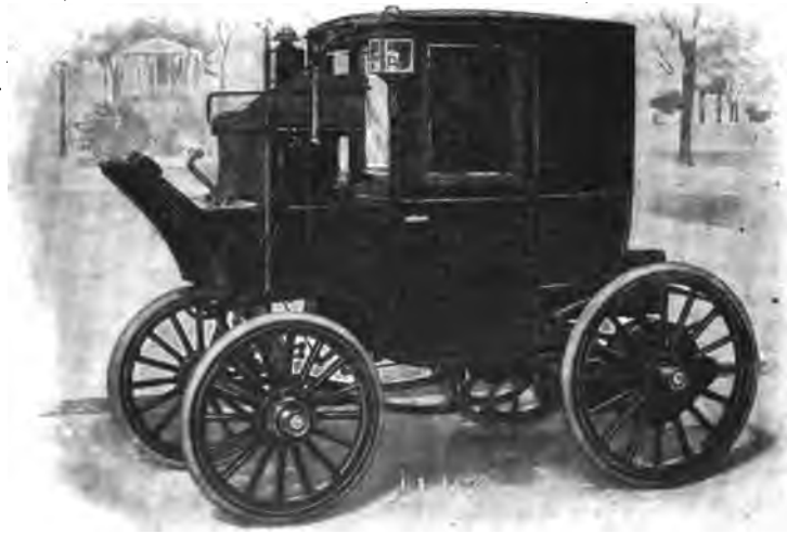
FIG. 439.—Square-front Brougham, Riker type, for city and general family service. The weight of this carriage is 4,000 pounds; travel radius per full charge of battery, thirty-five miles; maximum speed, twelve miles per hour.
